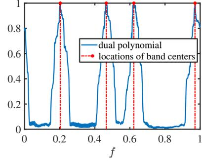
Figure 1. Dual polynomial  $\hat{q}(f)$  (see (9)) for multiband signal identification. Here, the dashed red lines represent the true frequencies, which are correctly localized by examining the peaks of the dual polynomial.
