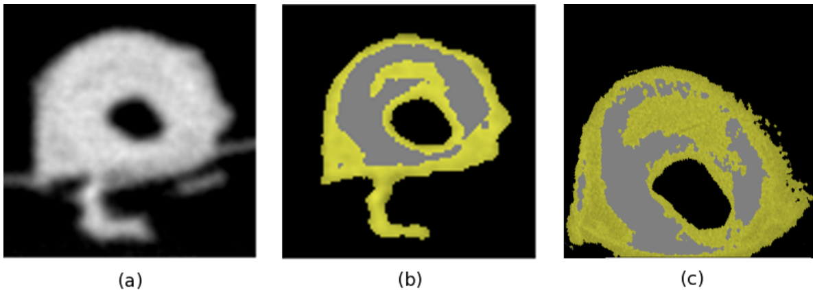
Fig. 6: Preliminary results from study of flat panel data. Shown are a) unprocessed flat panel data and b) colored flat-panel DTSA output. Panel c) shows the same sample, imaged by a \mu CT scanner and colored by the DTSA algorithm. The two data sets have been manually registered. For detail about these \mu CT results, see [4].
