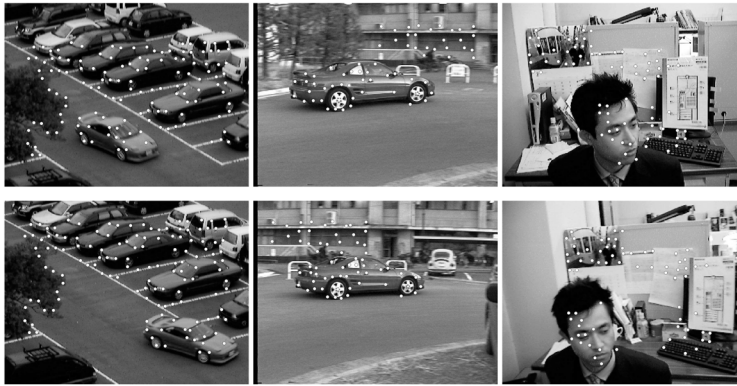
Fig. 9. Segmenting the point correspondences of sequences A (left), B (center), and C (right) in [14] for each pair of consecutive frames by segmenting subspaces in \mathbb{R}^5 . First row: first frame of the sequence with point correspondences superimposed. Second row: last frame of the sequence with point correspondences superimposed.
