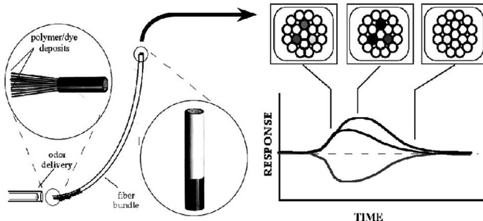
Fig. 10. The plot represents sensor/analyte signatures for three sensors within the bundled 19-sensor array. This figure was published in Nature 382 (1996) 697–700, and is reprinted by permission.
