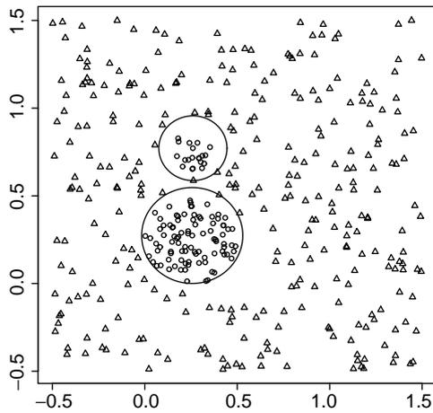
Fig. 3. Case I. The domain space class-conditional scatter plot ( $\mathcal{E} = \mathbb{R}^2$ ) and the algorithmically produced cover  $(\mathcal{W}, \mathcal{R})$  for the target class observations  $\mathcal{X}_J$  (represented by “o”s). The scale dimensional  $d^* = 2$ , and the cardinality  $c = 2$ ; a cover with two fundamental scales and two witness elements yields  $\hat{L}_J^{(R)} = 0$ .
