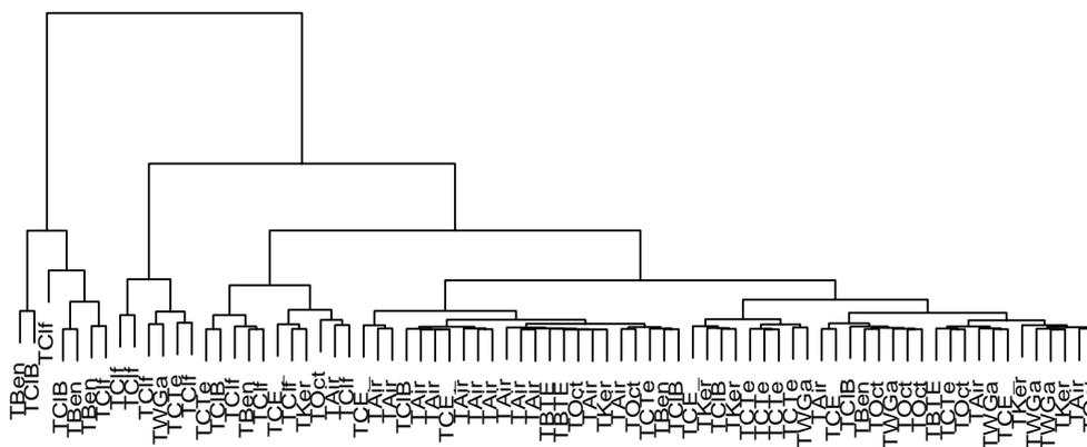
Fig. 12. Cluster tree for the Tufts artificial nose, after pruning at  $p = 5$ . (The cardinality  $c_5 = 76$ .) The leaf label indicates the chemical content of the observation.
