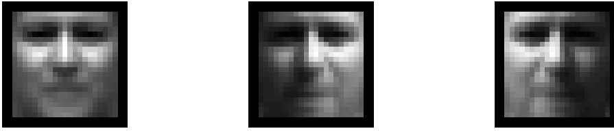
Figure 11. Clusters found by the CCCD classifier while training a boosted tree classifier. Each image represents the mean face within that cluster. While the clusters are ultimately chosen to maximize classification performance, they do correspond to the major image classes that are intuitively expected. Frontal, left and right illumination are all the dominant clusters.
