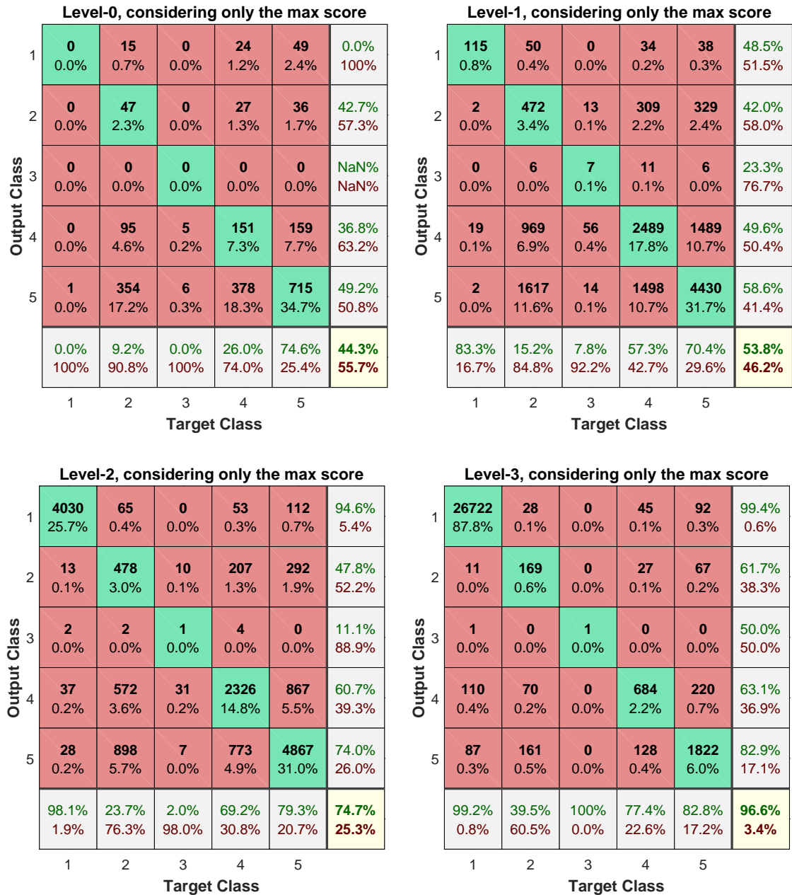
Figure 5.8: CatNet confusion matrix on the “test” set broken down for different levels of resolution when classification is only based on the top score.
