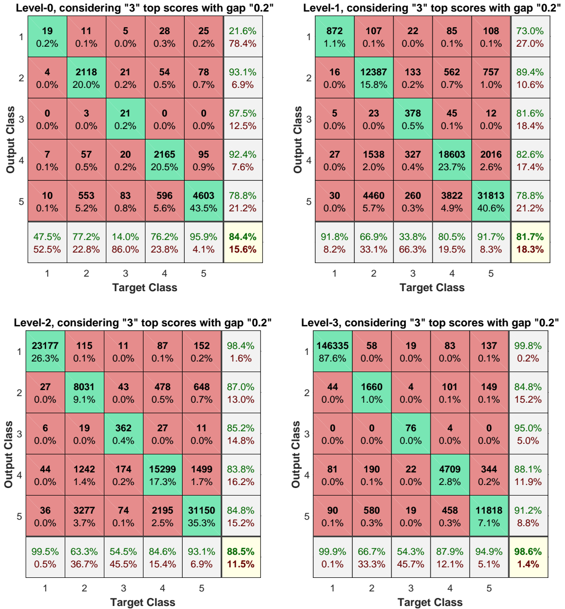
Figure E.3: CatNet confusion matrix on the “training” set broken down for different levels of resolution when classification is based on the top-3 scores and score gap 0.2.
