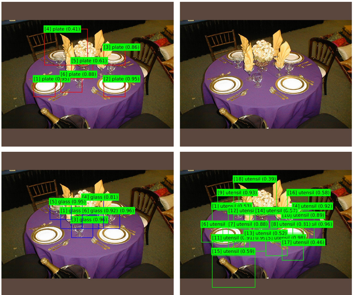
Figure 5.19: CNN classifier detections for “plate” (top left), “bottle” (top right), and “glass” (bottom left), and “utensil” (bottom right) categories. The ordinal numbers in brackets represent the confidence rank of detections per category and the fractional values in parentheses indicate the scale ratio of detections.
