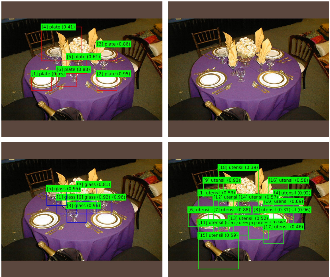
Figure 6.16: CNN detections for “plate” (top left), “bottle” (top right), and “glass” (bottom left), and “utensil” (bottom right) categories. The ordinal numbers in brackets represent the confidence rank of detections per category.
