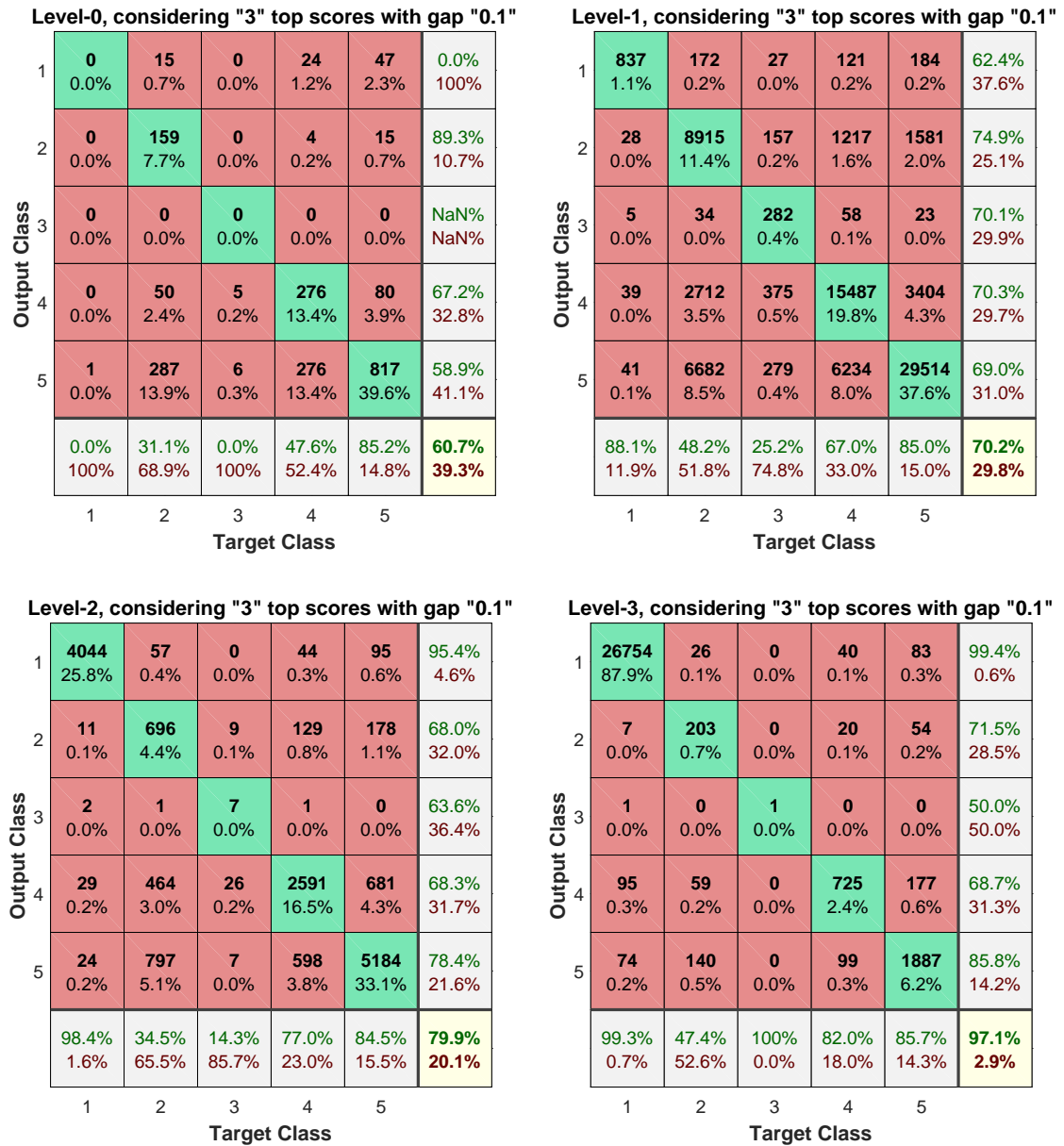
Figure 5.9: CatNet confusion matrix on the “test” set broken down for different levels of resolution when classification is based on the top-3 scores and score gap 0.1.
