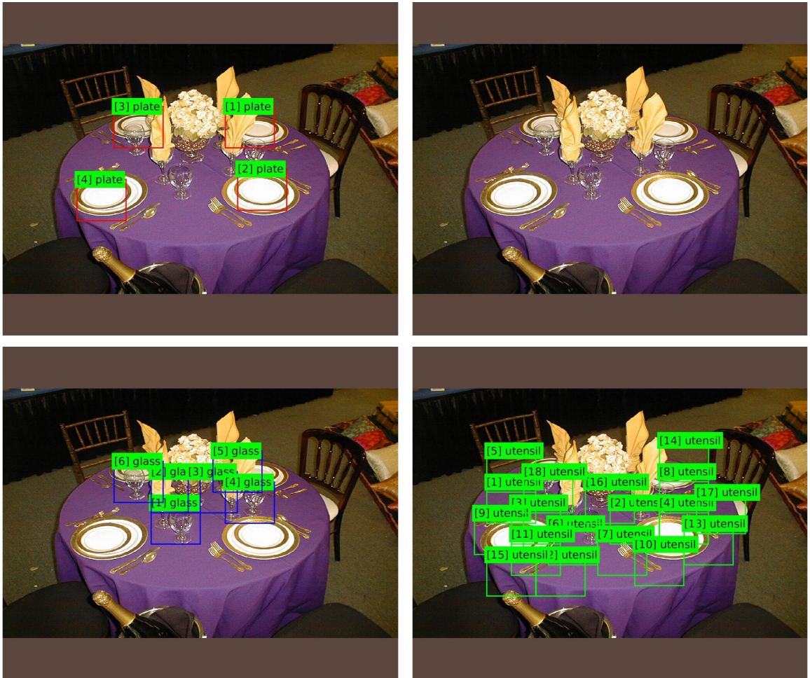
Figure 6.14: Model-based detections (all questions) for “plate” (top left), “bottle” (top right), and “glass” (bottom left), and “utensil” (bottom right) categories. The ordinal numbers in brackets represent the confidence rank of detections per category.
