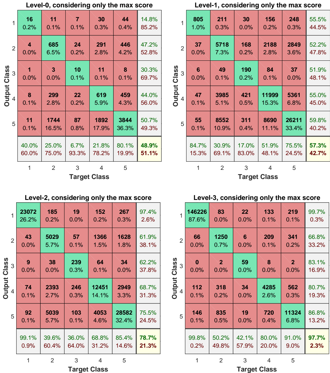
Figure E.1: CatNet confusion matrix on the “training” set broken down for different levels of resolution when classification is only based on the top score.
