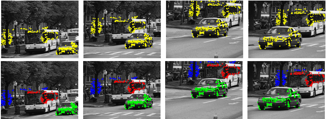
Figure 3.1: Motion segmentation: given feature points on multiple rigidly moving objects tracked in multiple frames of a video (top), the goal is to separate the feature trajectories according to the moving objects (bottom).
