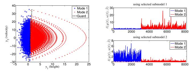
Fig. 2. Left: height-velocity graph using the ground-truth discrete modes and the separating hyperplane learned by our proposed algorithm. Right: representation error of the data using the two submodels selected by our algorithm from the set of estimated models. The observation indices on the horizontal axis are reordered such that the first 3079 indices correspond to mode 1, while the next 5021 indices correspond to mode 2.
