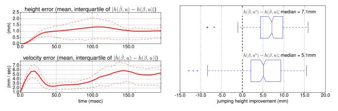
Fig. 3. Control of jumping robot using estimated model. *Left:* prediction error. *Right:* jumping height improvement.
