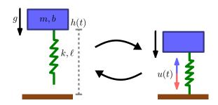
Fig. 1. Illustration of the jumping robot from Section 4. *Left:* mass moves vertically in a gravitational field. *Right:* actuator and leg spring exert forces on the mass when the leg spring is in contact with the ground.
