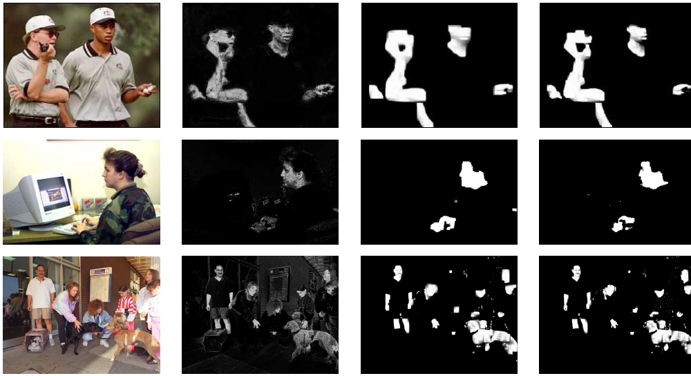
Fig. 4. First column: original color images. The image on top is 225 \times 180 pixels . The image on the bottom is 541 \times 361 pixels. Second column: Baseline model. Third column: hidden Markov model. Fourth column: First Order Model. In the computed images, the grey level is proportional to the skin probability evaluated with the specified model.
