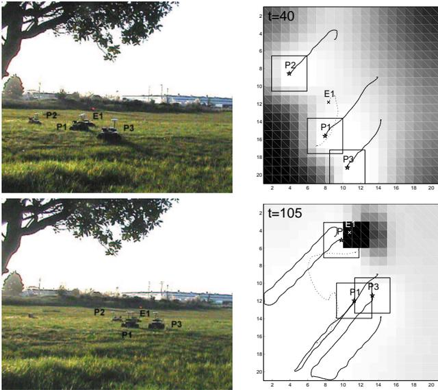
Fig. 3. Experiment 1: An actual game between 3 UGV pursuers and 1 UGV evader. The pursuers P1, P2 and P3 (\*) move at 0.3 m/s and use the global-max policy with an omni-directional visibility region. The evader E1 moves randomly at 0.1 m/s.
