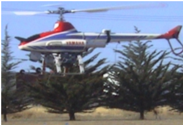
Figure 5: UAV based on Yamaha R-50 Helicopter
